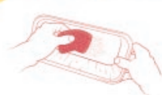
Roughen the inside of the larger loaf pan using sandpaper or steel wool. Do the same to the outside of the smaller aluminum loaf pan.
