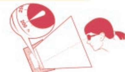
Wearing sunglasses, monitor the temperature inside the oven. Allow the oven to reach 200°C (350°F or higher) to burn off unwanted materials in the paint and glue.
