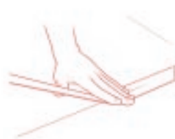
Apply tape to join panels. TIP —So that you can later fold them at the join, allow a small space (3 mm) between sections before taping.
