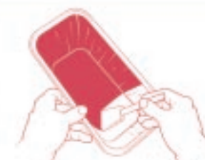
Apply 2 coats of black paint and glue mixture to the inside of the large aluminum loaf pan.
