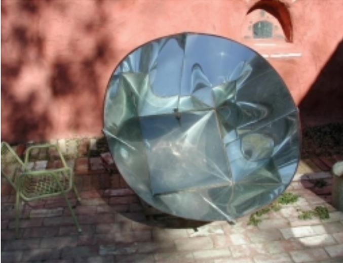
A parabolic reflector can produce extremely high temperatures when aimed at the sun.
