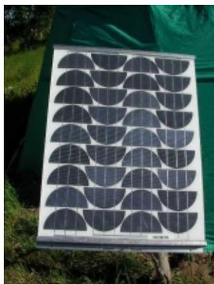
Many single photovoltaic cells are connected by wires and mounted on a flat panel to form a photovoltaic array.
