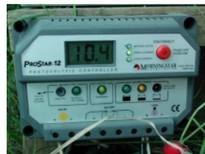
An electronic charge controller used to maintain the health of a rechargeable battery connected to a solar panel.
